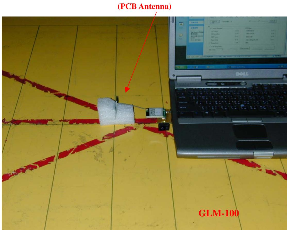
**Photo 4: Radiated Emission Test set-up photo**
