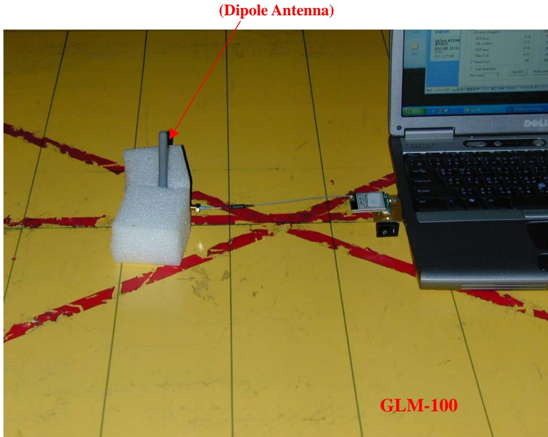
**Photo 2: Radiated Emission Test set-up photo**
