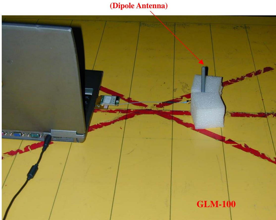
**Photo 3: Radiated Emission Test set-up photo**
