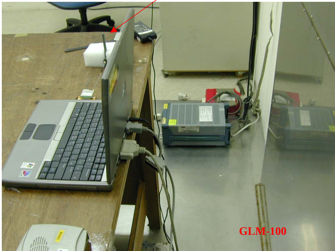
Photo 2: Conducted Emission Test set-up photo (Dipole Antenna)
