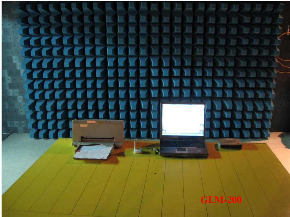
Photo 1: Radiated Emission Test set-up photo Dipole antenna
