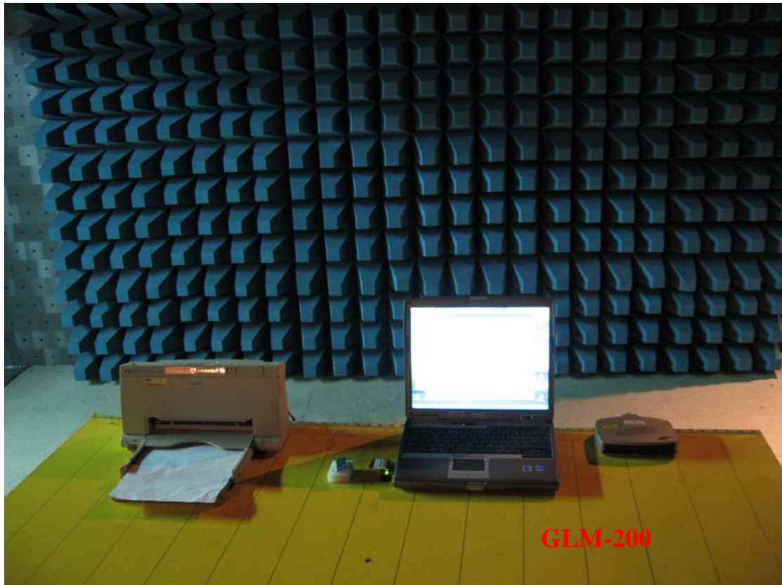
Photo 3: Radiated Emission Test set-up photo PCB antenna
