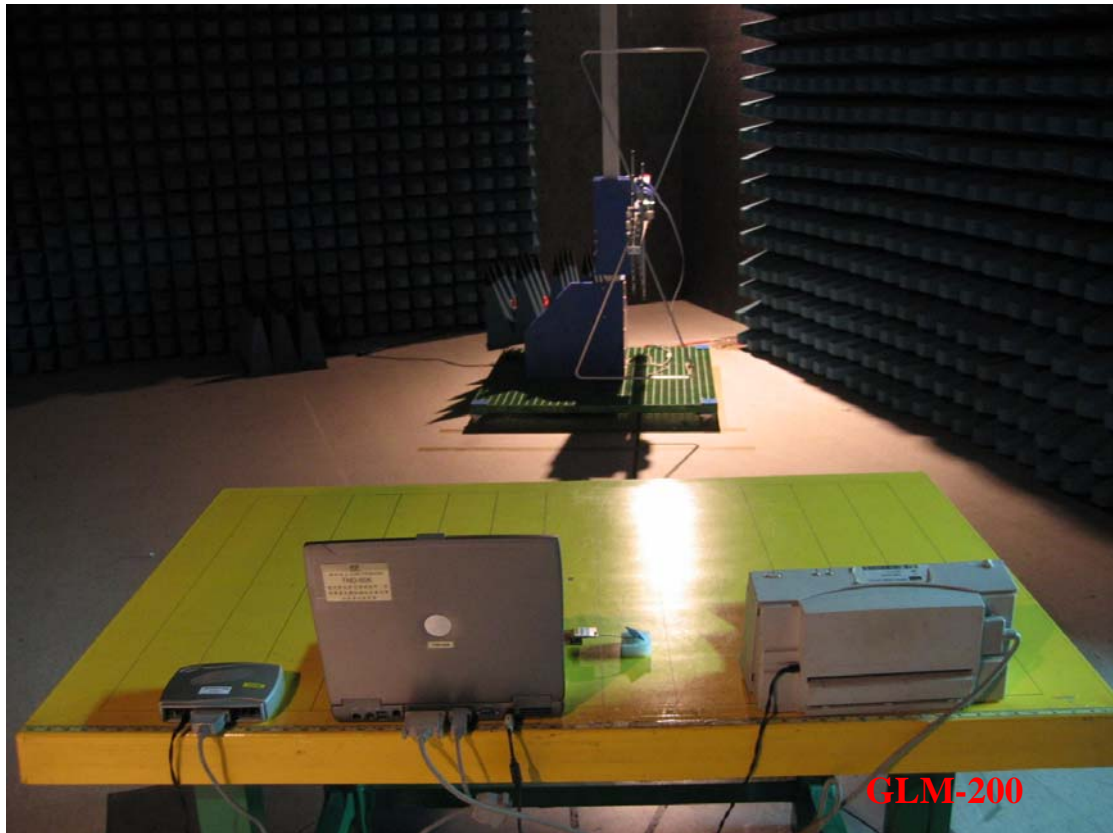
Photo 4: Radiated Emission Test set-up photo PCB antenna
