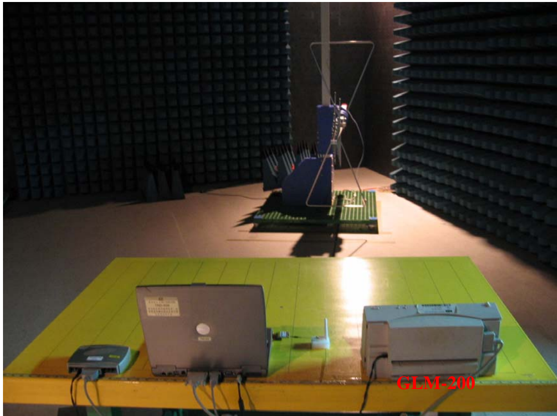
Photo 2: Radiated Emission Test set-up photo Dipole antenna
