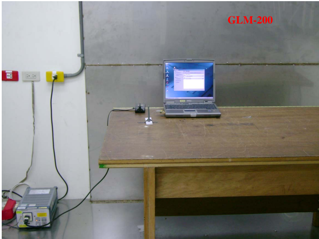
Photo 1: Conducted Emission Test set-up photo
