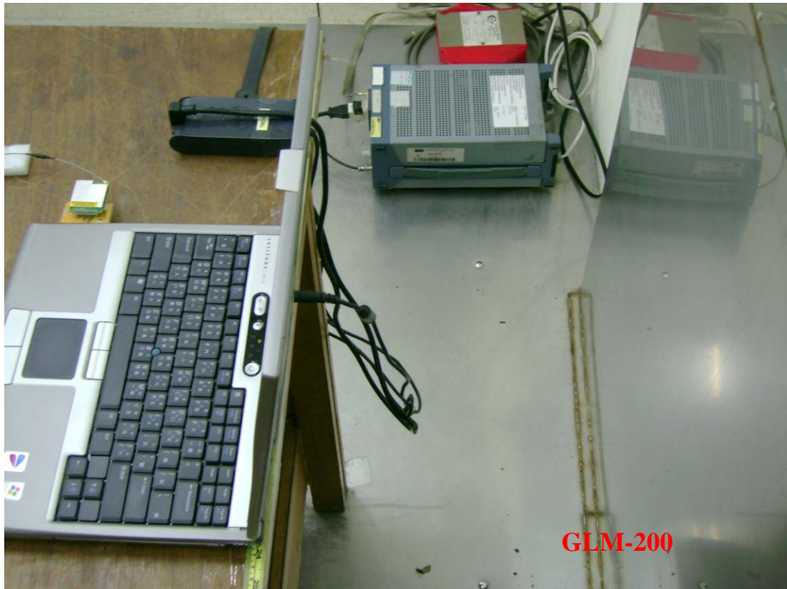
Photo 2: Conducted Emission Test set-up photo
