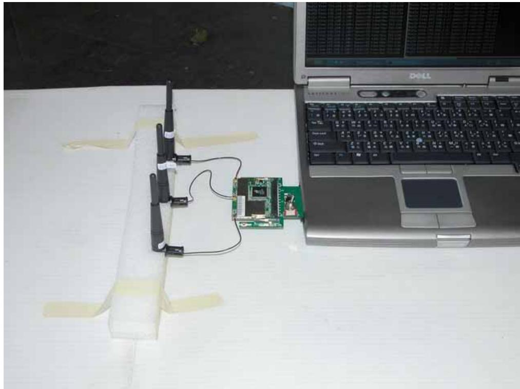
**RADIATED RF MEASUREMENT SETUP**
