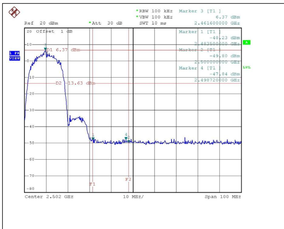
The spectrum plots are attached on the following page. D1 line indicates the highest level, D2 line indicates the 20dB offset below D1. It shows compliance with the requirement in part 15.247(C).
