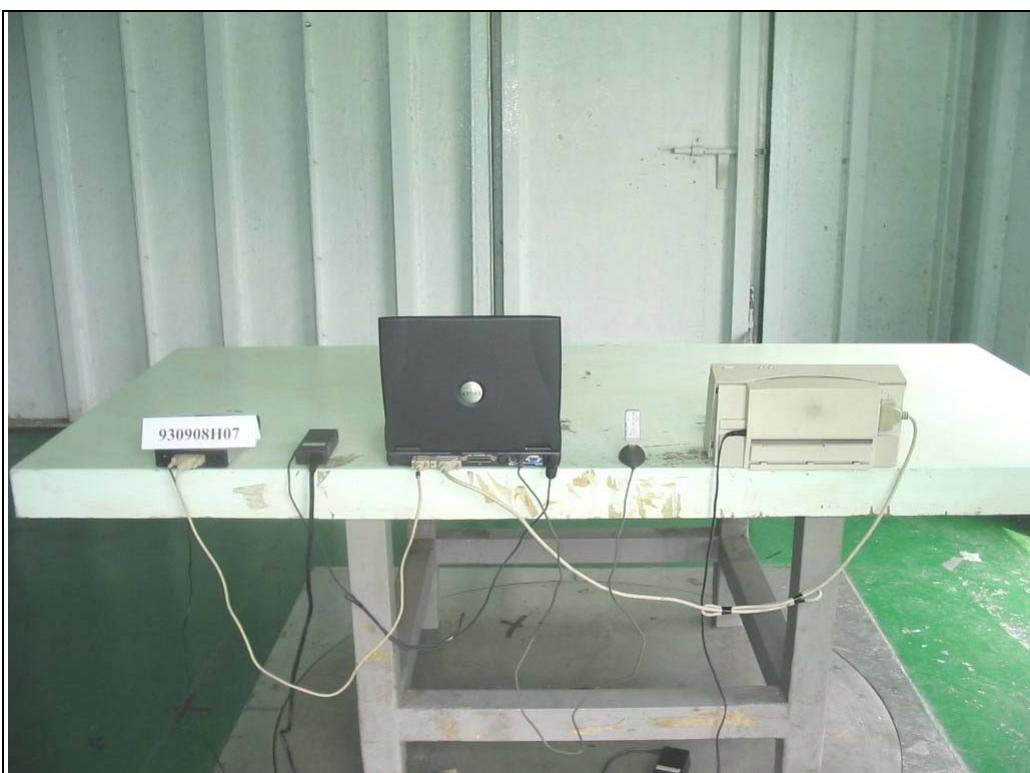
RADIATED EMISSION TEST (Without USB Cable)
