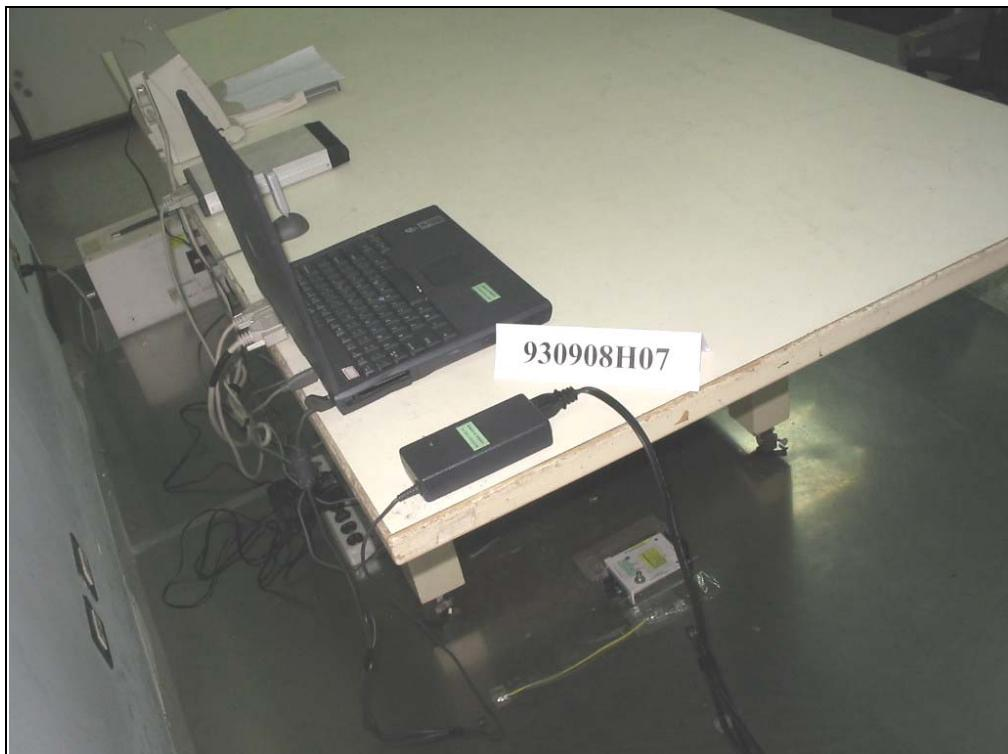
CONDUCTED EMISSION TEST (Without USB Cable)
