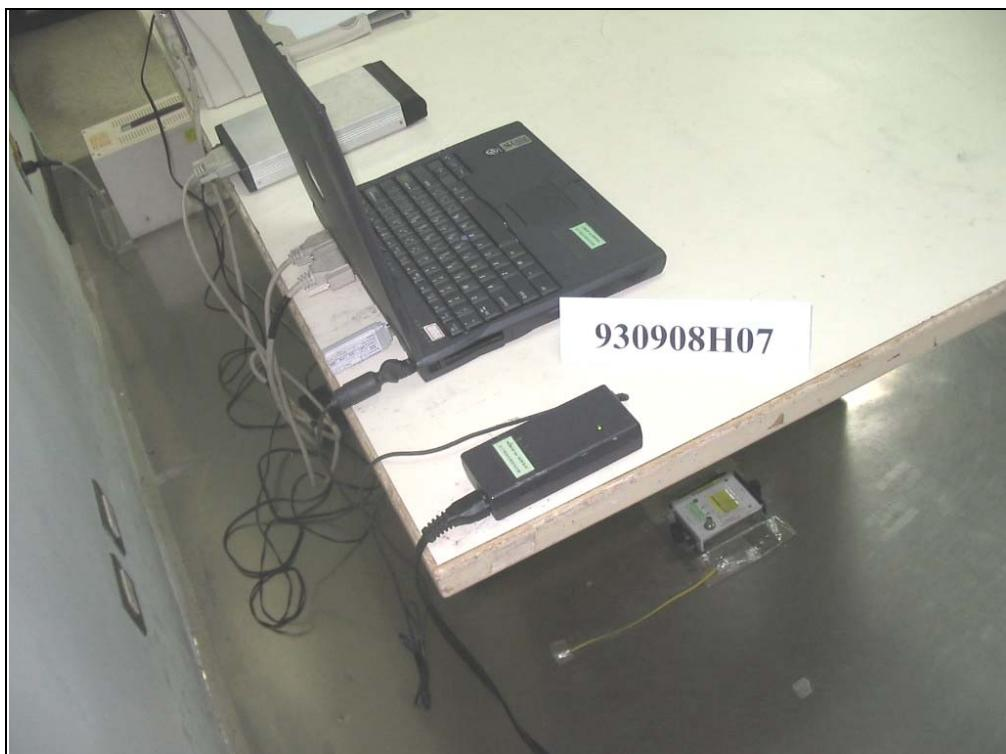
RADIATED EMISSION TEST (With USB Cable)
