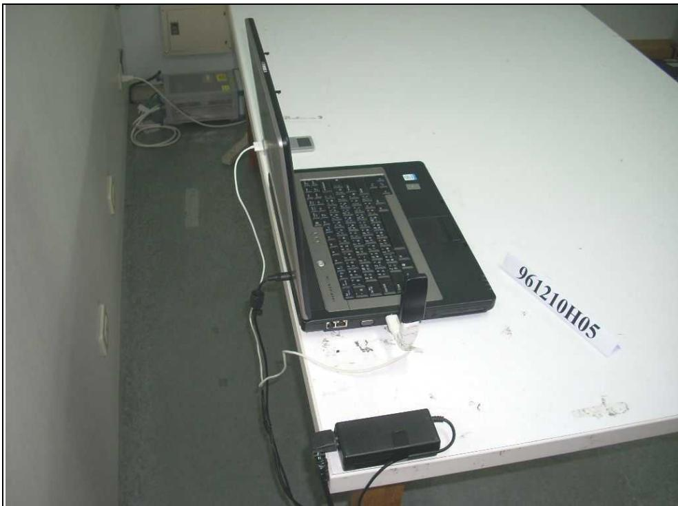
RADIATED EMISSION TEST – with 1.5m USB cable
