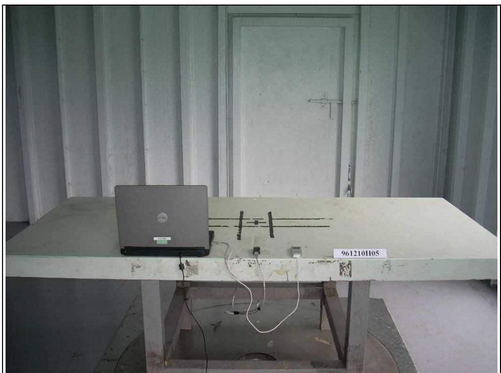
RADIATED EMISSION TEST – with 0.15m USB cable
