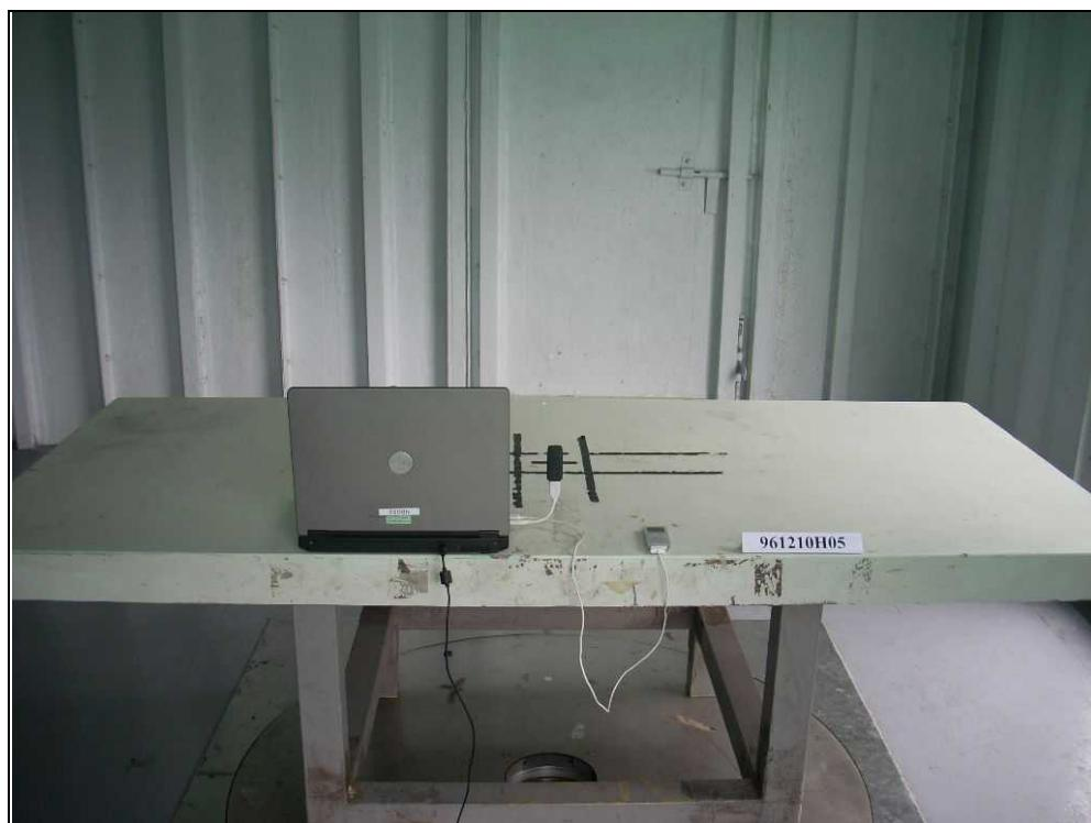
RADIATED EMISSION TEST – without USB cable
