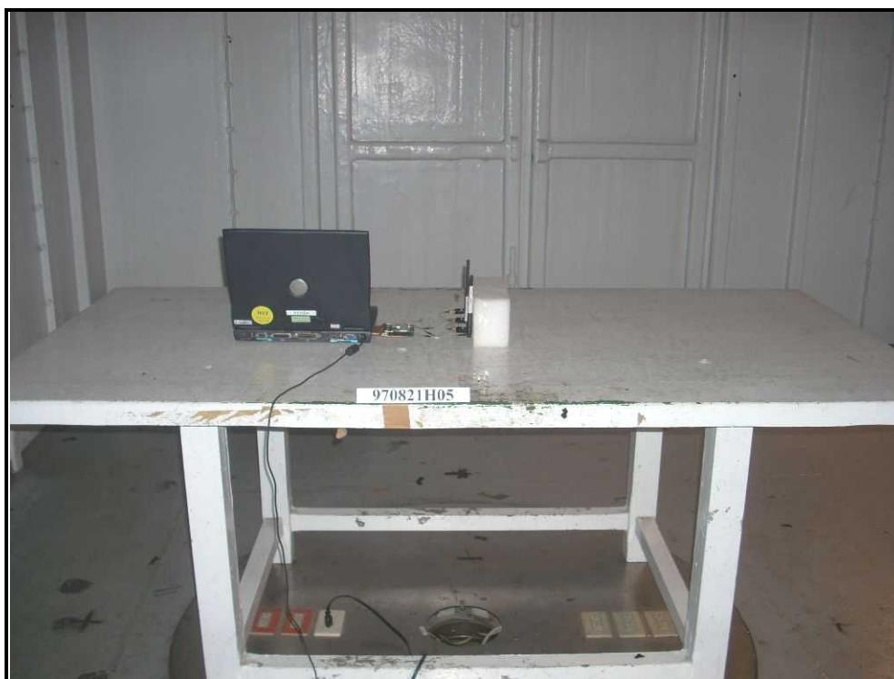
RADIATED EMISSION TEST – Site C (Dipole antenna)
