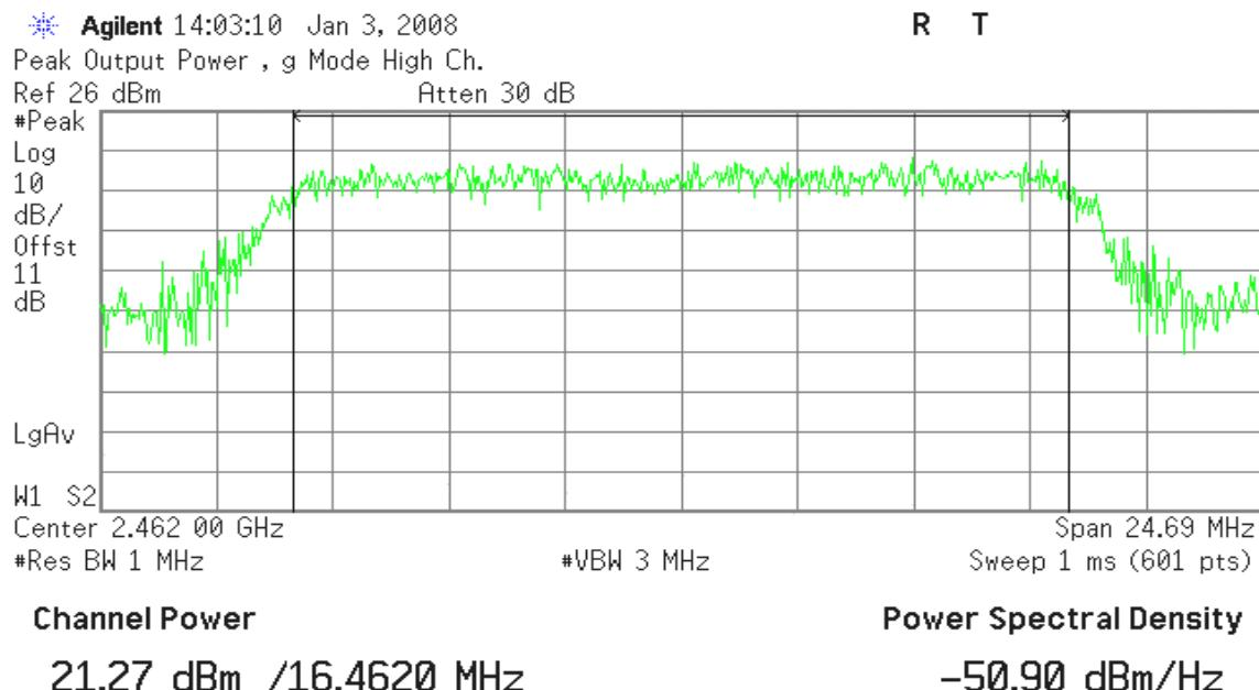
**draft 802.11n Standard-20 MHz Channel mode****Peak Power (CH Low)**
