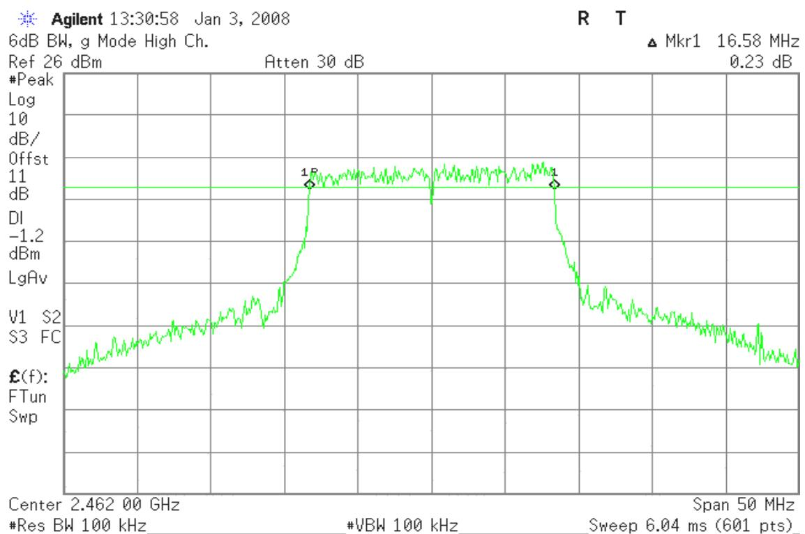
**draft 802.11n Standard-20 MHz Channel mode****6dB Bandwidth (CH Low)**
