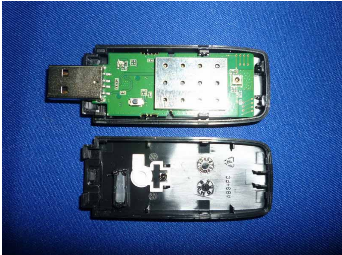
Figure 4 Inside of the EUT
