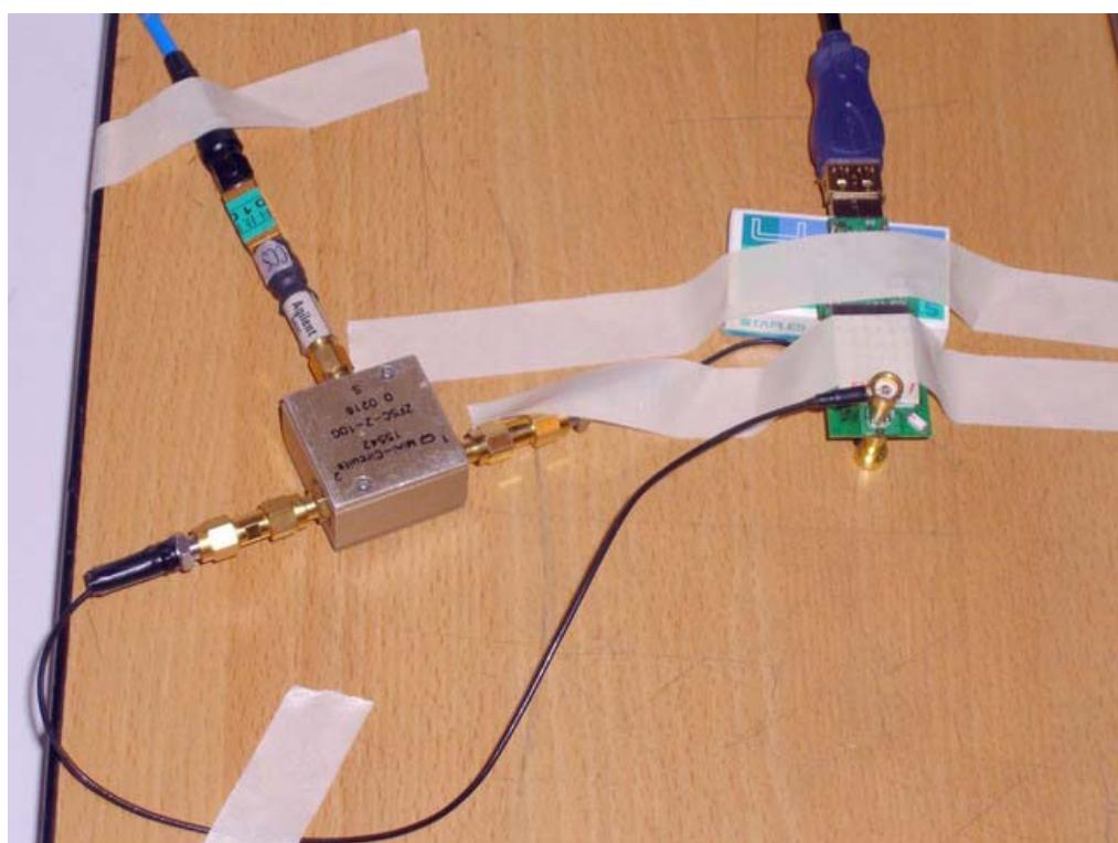
**POWERLINE CONDUCTED EMISSIONS MEASUREMENT SETUP**
