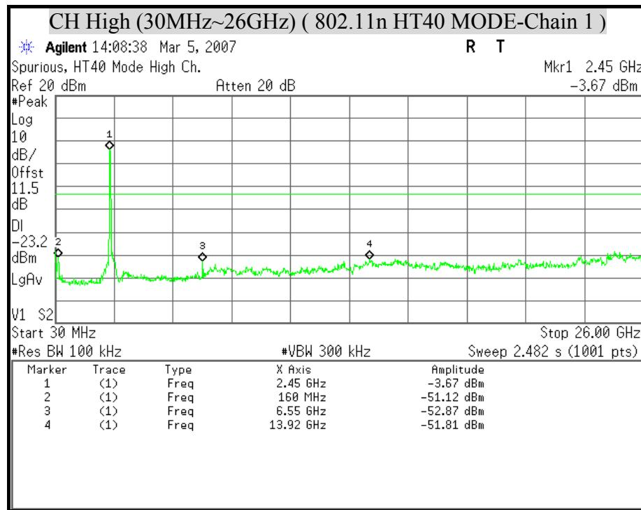
**OUT-OF-BAND SPURIOUS EMISSIONS-CONDUCTED MEASUREMENT****( 802.11n HT40 Combined MODE )**
