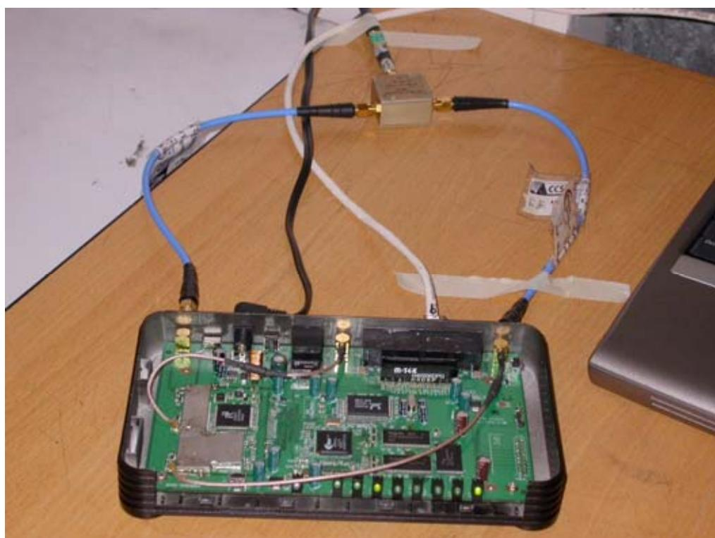
**POWERLINE CONDUCTED EMISSIONS MEASUREMENT SETUP**
