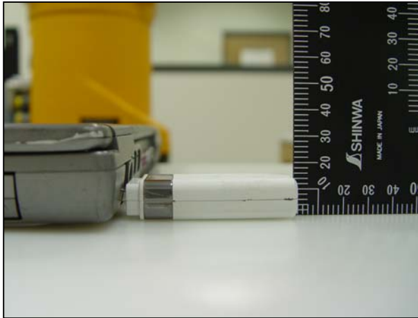
Distance is 0mm for Bottom Face Touch
