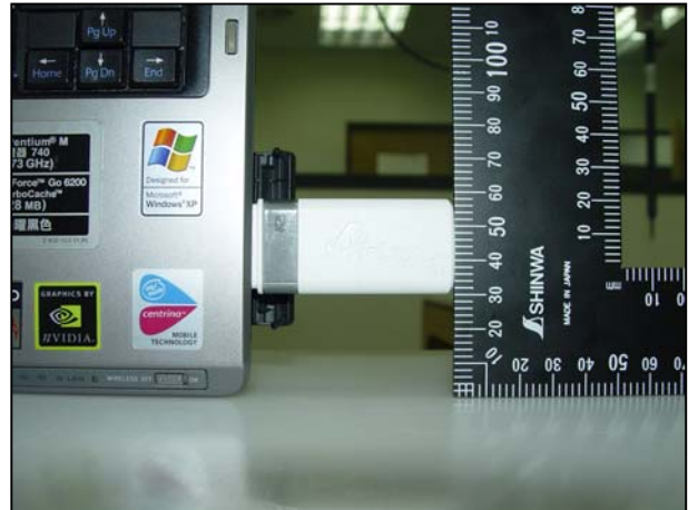
Distance is 30mm for Side(Edge) Touch
