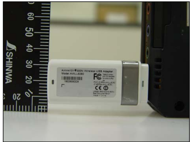
Distance is 6mm for Side(Edge) Touch
