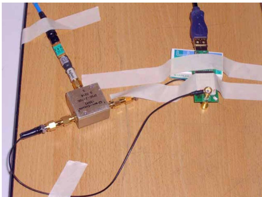
**POWERLINE CONDUCTED EMISSIONS MEASUREMENT SETUP**
