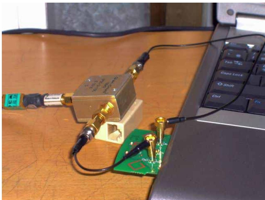
**POWERLINE CONDUCTED EMISSIONS MEASUREMENT SETUP**
