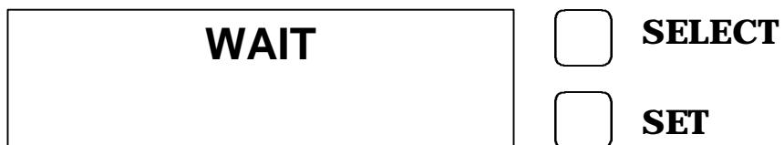
After 3 seconds the green PLL LOCK led will light and the Display will show an increasing bar, after a further 5 seconds the green ON AIR led will light and there will be output power.
