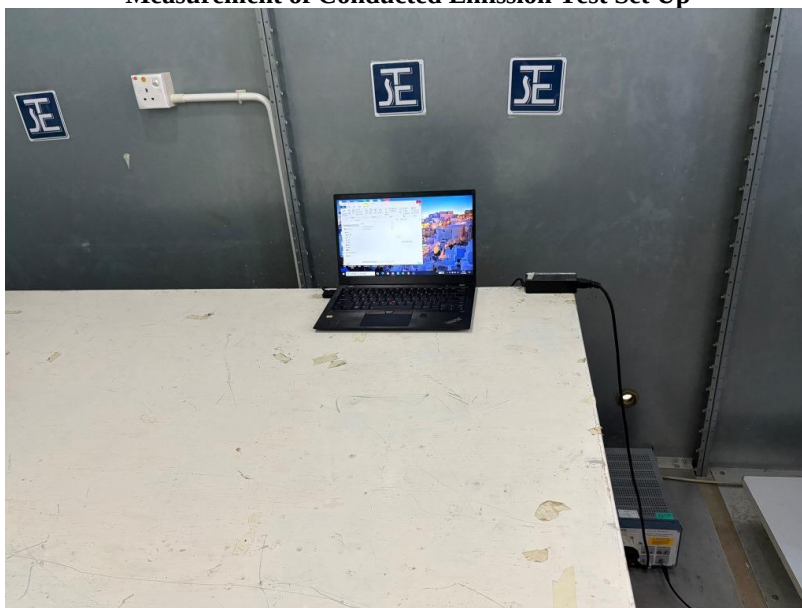
Measurement of Conducted Emission Test Set Up
