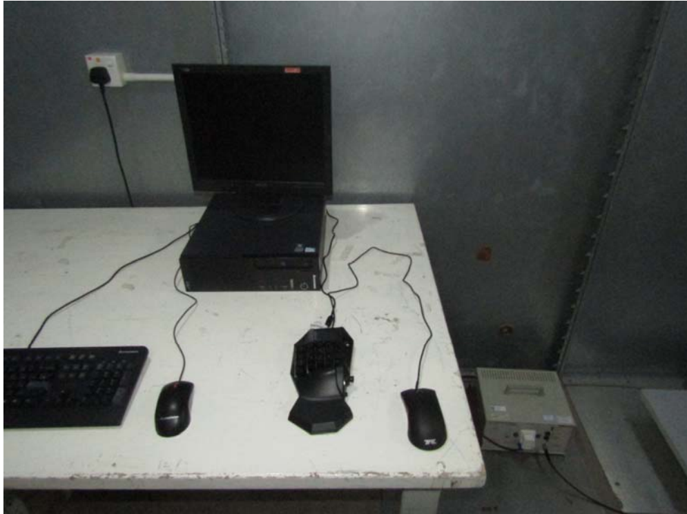
Measurement of Conducted Emission Test Set Up
