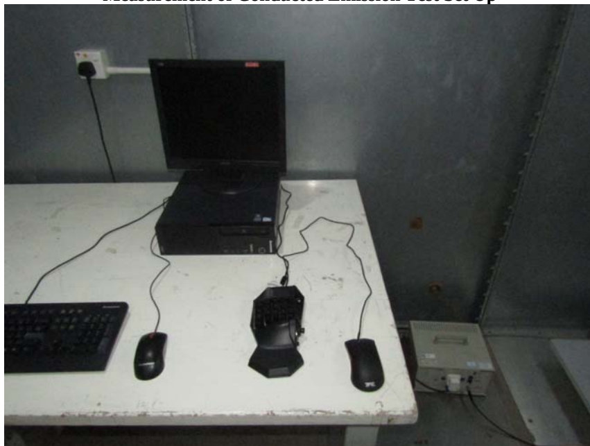
Measurement of Conducted Emission Test Set Up
