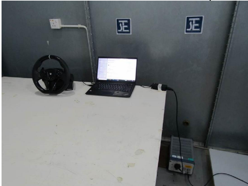
Measurement of Conducted Emission Test Set Up
