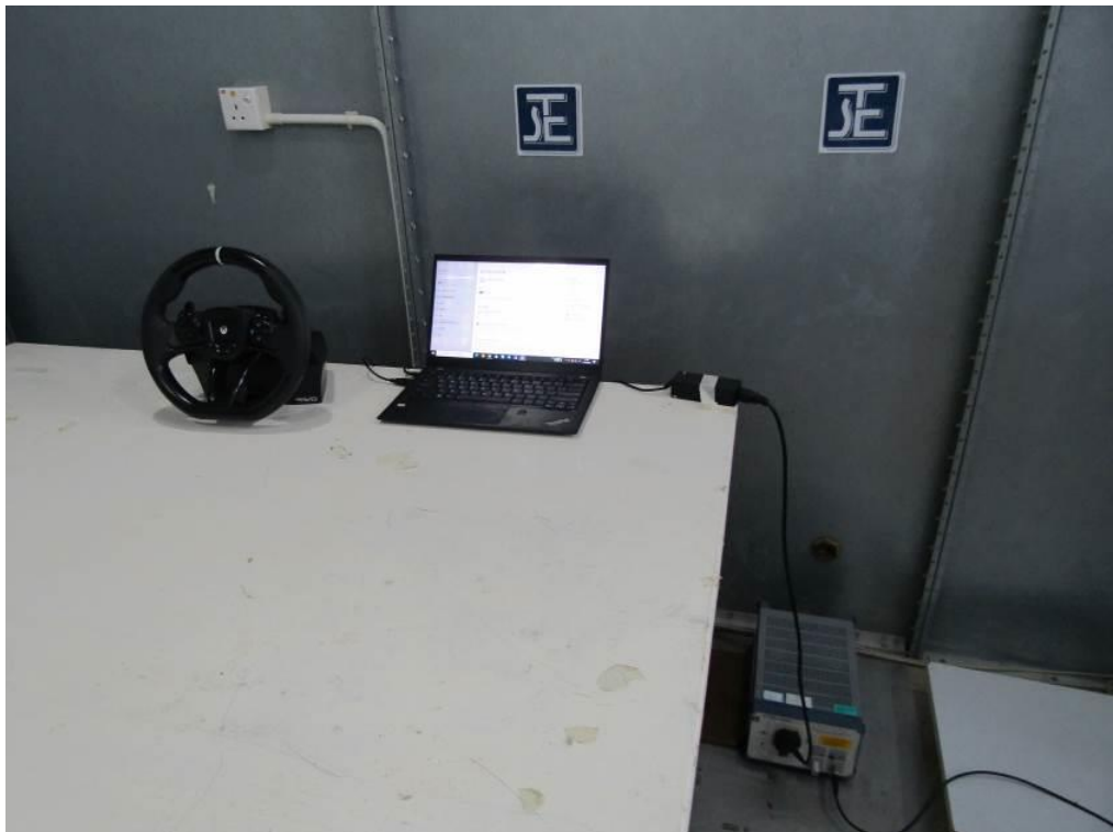
Measurement of Conducted Emission Test Set Up
