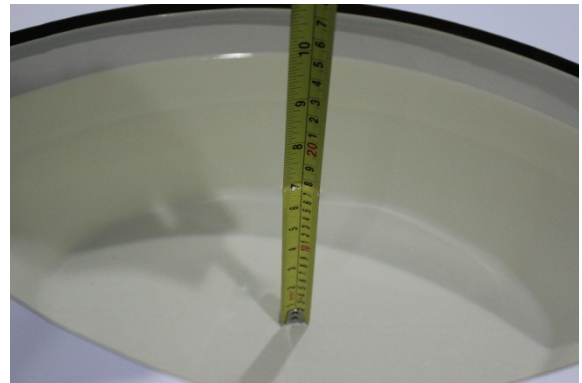
Liquid depth in the body phantom (2600MHz)
