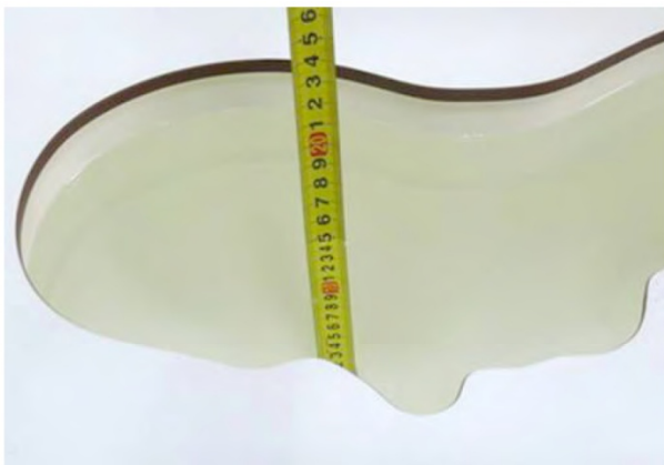
Liquid depth in the head phantom (1900MHz)
