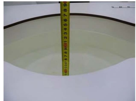
Liquid depth in the body phantom (1900MHz)
