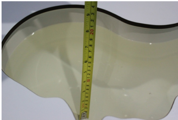
Liquid depth in the head phantom (2600MHz)
