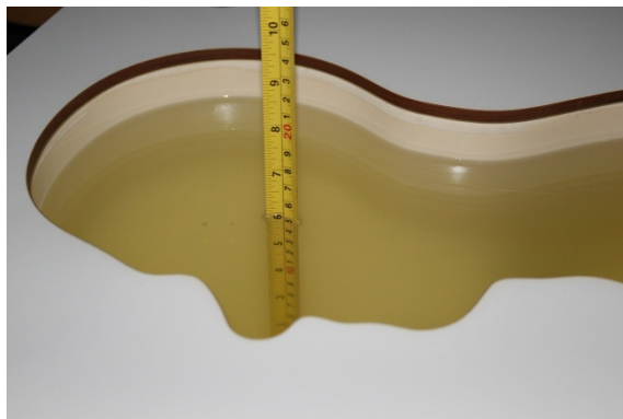
Liquid depth in the head phantom (1750MHz)
