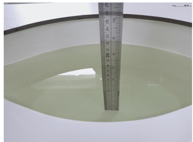
Liquid depth in the body phantom (2450MHz)
