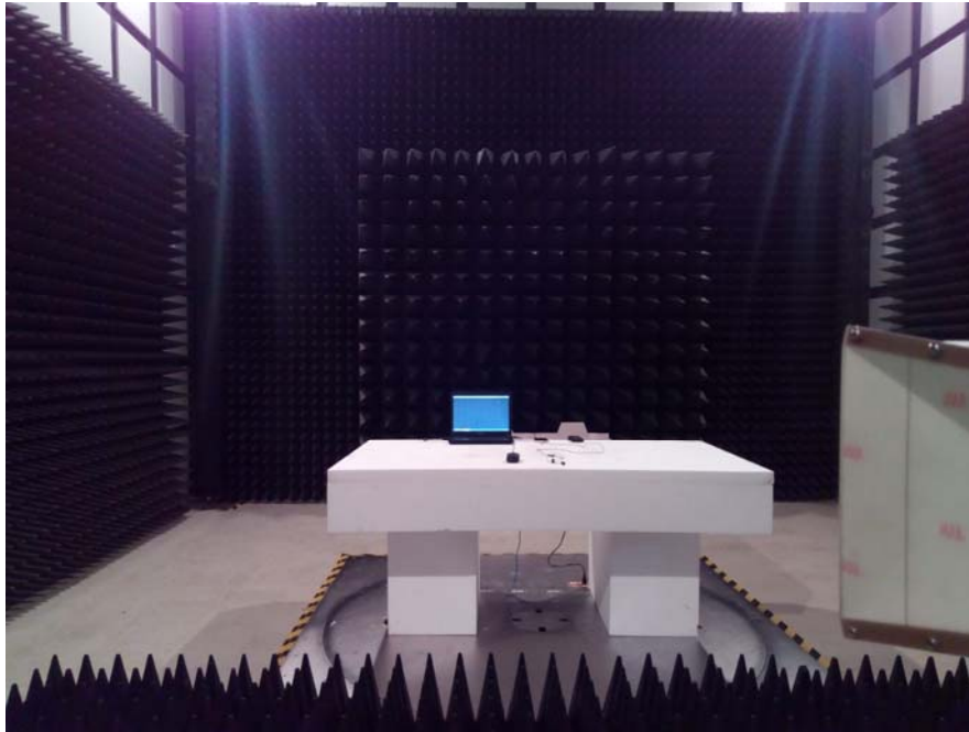
Radiated Emissions – Front View (Above 1 GHz)
