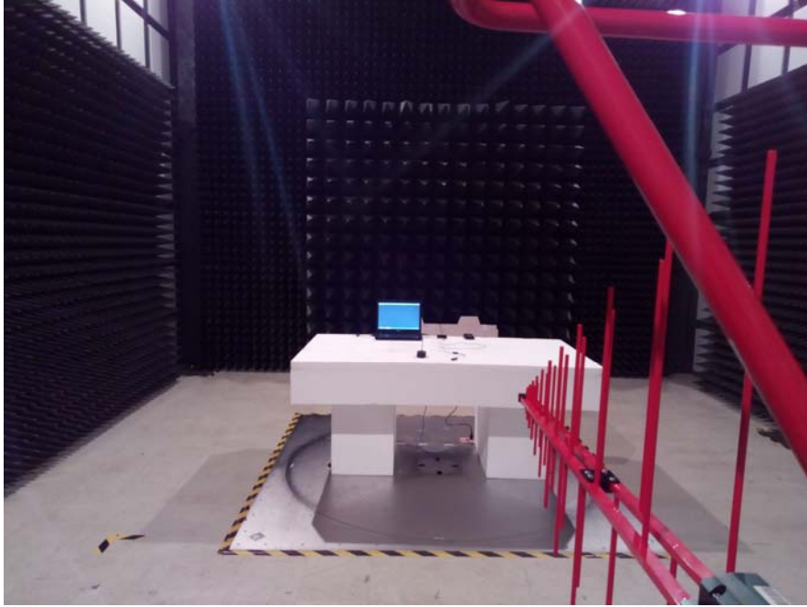
Radiated Emissions – Front View (Below 1 GHz)
