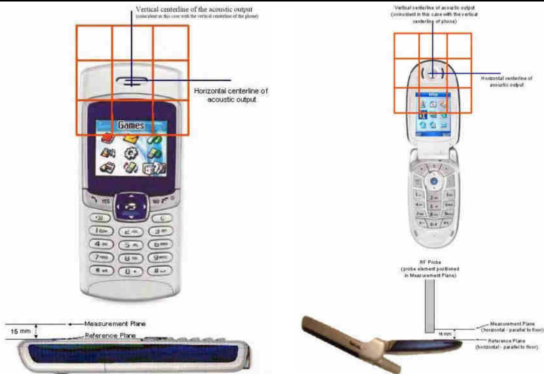
Fig 7.2 EUT reference and plane for HAC RF emission measurements
