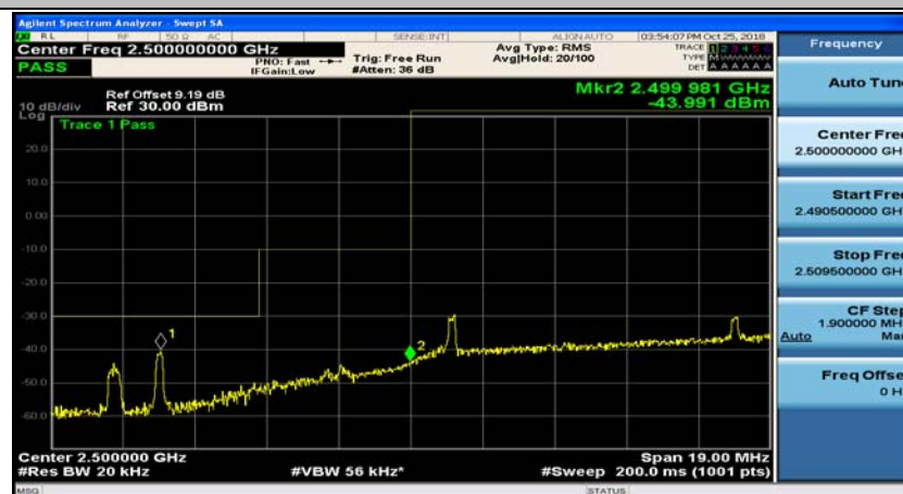
(Channel Bandwidth:20 MHz)_LCH_QPSK_50RB#0
