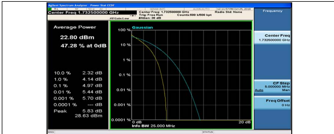
(Channel Bandwidth:20 MHz)_MCH_QPSK_100RB#0
