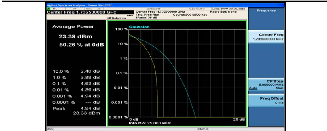
(Channel Bandwidth:15 MHz)_MCH_QPSK_1RB#74
