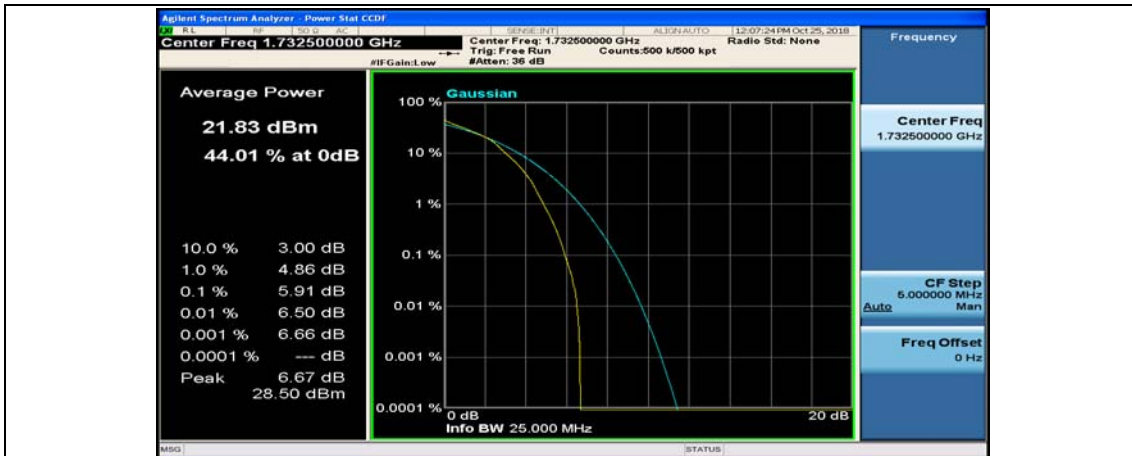
(Channel Bandwidth:15 MHz)_MCH_16QAM_75RB#0
