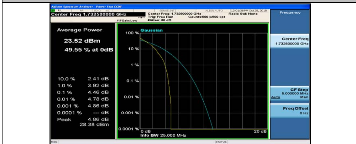
Channel Bandwidth: 10 MHz_MCH_QPSK_1RB#49
