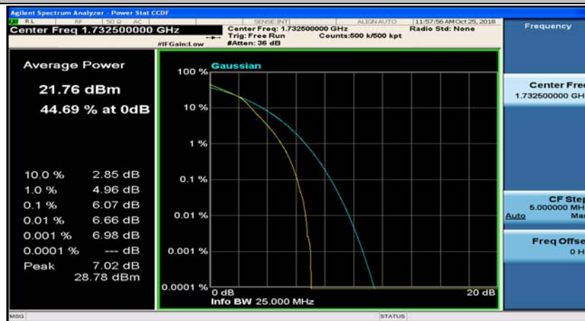
(Channel Bandwidth: 5 MHz)_MCH_16QAM_12RB#6
