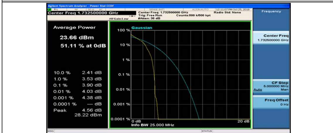
(Channel Bandwidth:20 MHz)_MCH_QPSK_1RB#49
