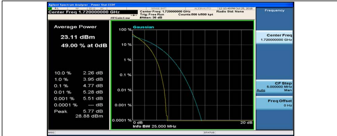
(Channel Bandwidth:20 MHz)_MCH_QPSK_1RB#0
