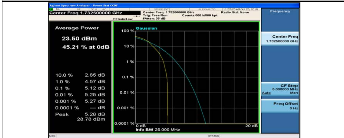
(Channel Bandwidth: 5 MHz)_MCH_16QAM_1RB#24
