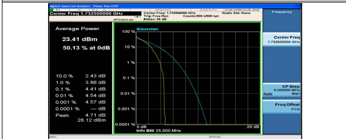
(Channel Bandwidth:15 MHz)_MCH_QPSK_1RB#37
