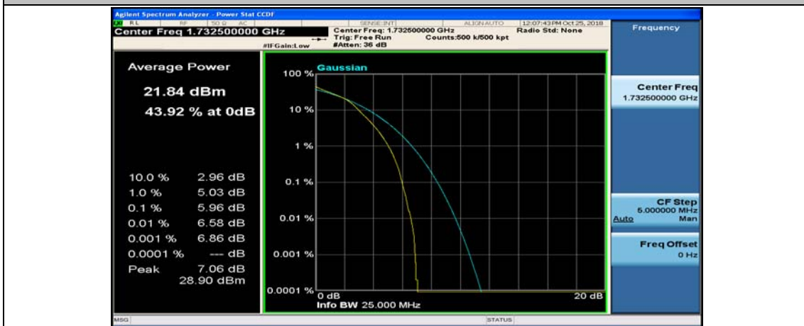
(Channel Bandwidth:15 MHz)_MCH_16QAM_75RB#0
