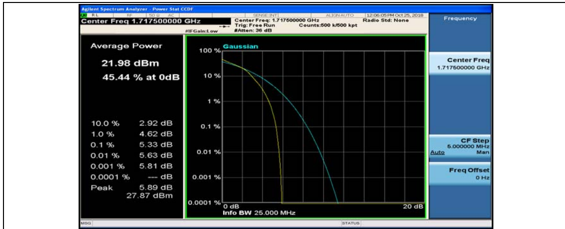
(Channel Bandwidth:15 MHz)_MCH_16QAM_1RB#0
