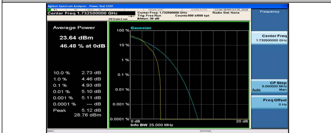
(Channel Bandwidth:15 MHz)_MCH_16QAM_1RB#74
