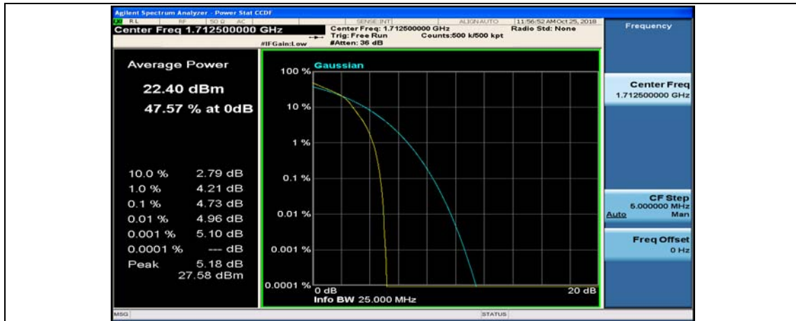
(Channel Bandwidth: 5 MHz)_MCH_16QAM_1RB#0
