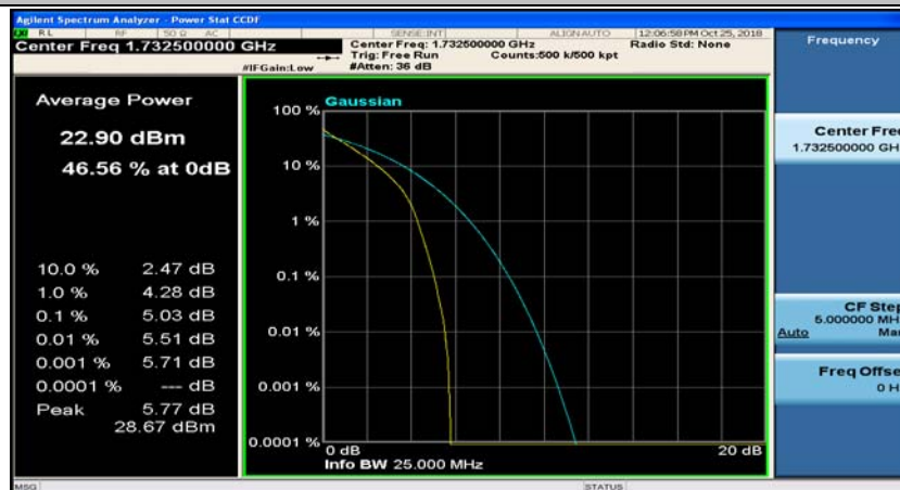
(Channel Bandwidth:15 MHz)_MCH_QPSK_37RB#38
