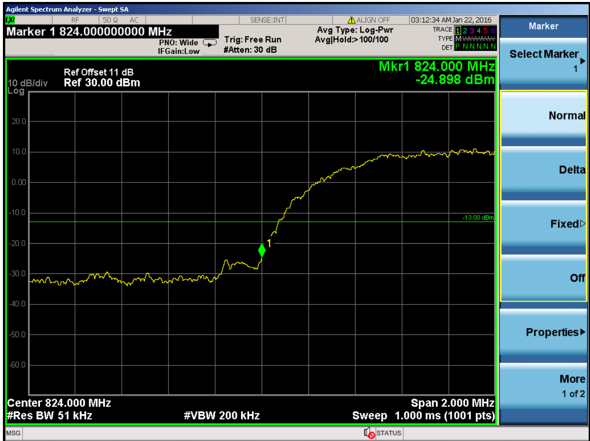
(Plot 4.5.2 A: Channel 4132: 826.4MHz @ WCDMA Band V)
