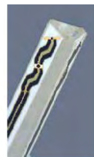
Figure 3.3 PROBE THICK-FILM TECHNIQUE
