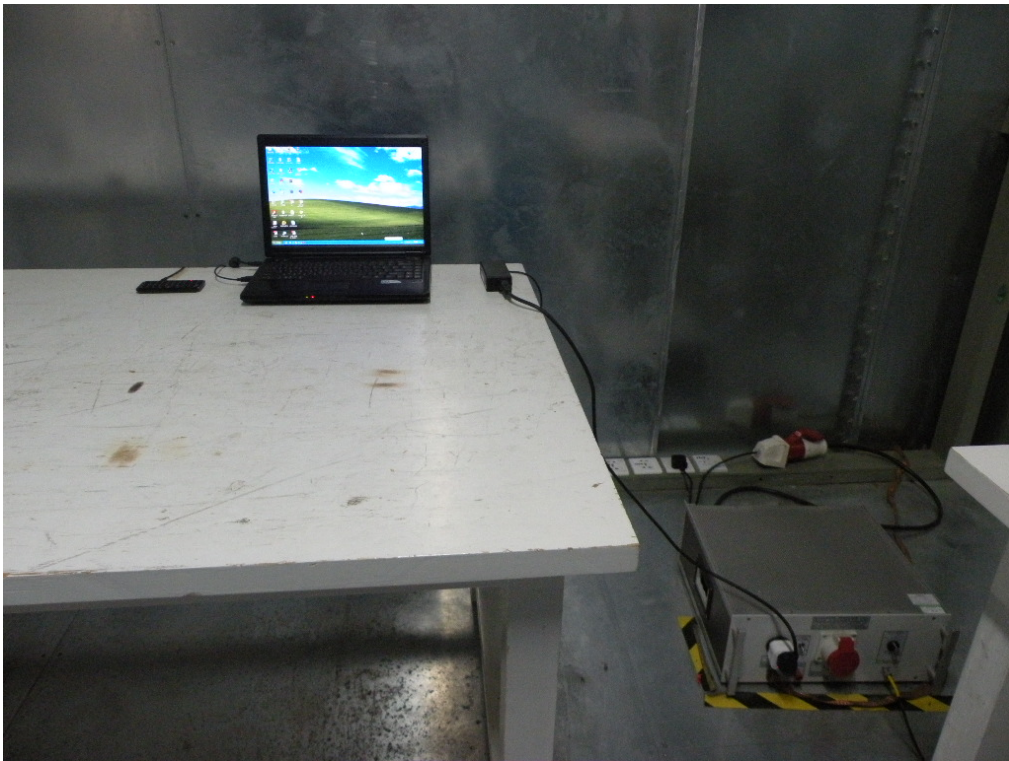
Radiated Emission Test Setup in Chamber
