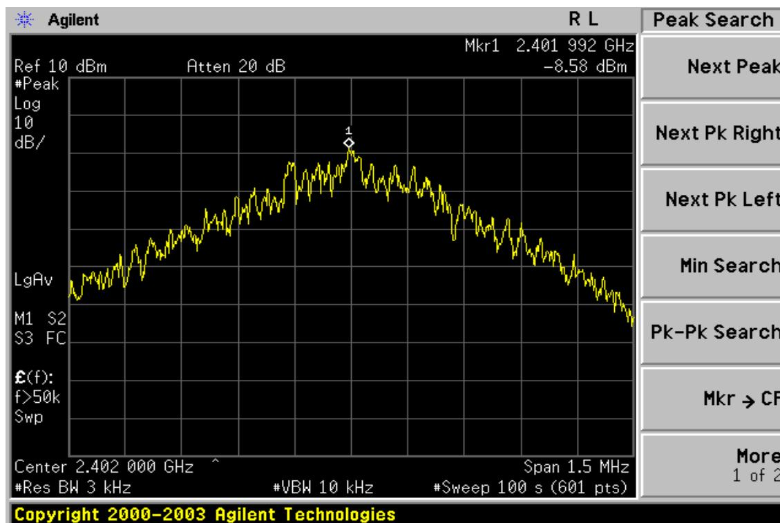
**Power Spectral Density Test Plot (CH-Mid)**
