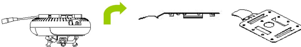
As the direction of picture shown above, put and slide the case on Mount Bracket which was already fixed on ceiling, pushing it carefully until you hear clear metallic sound, "TIC".
