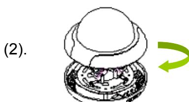
Turn Glass Cover to counter-clockwise direction to open the case and verify visually whether cameras in it are correctly connected.
