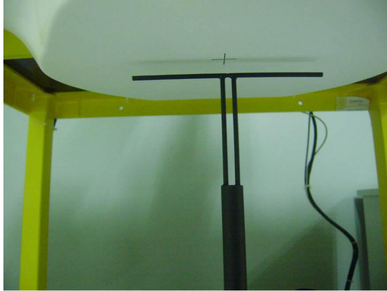
Fig 7.2 Setup Photo of Dipole Antenna
