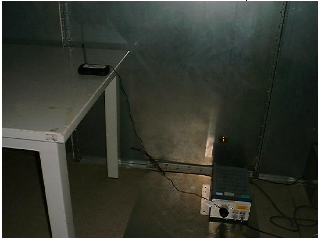
Measurement of Conducted Emission Test Set Up
