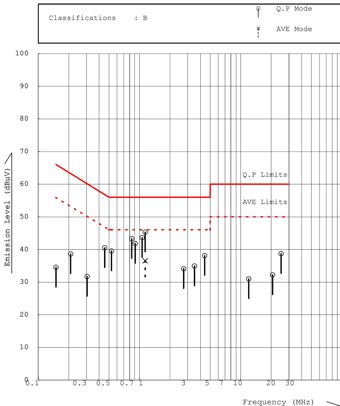
**2.1.4. AC Powerline Conducted Emission Measurements (0.15 MHz - 30 MHz)**
