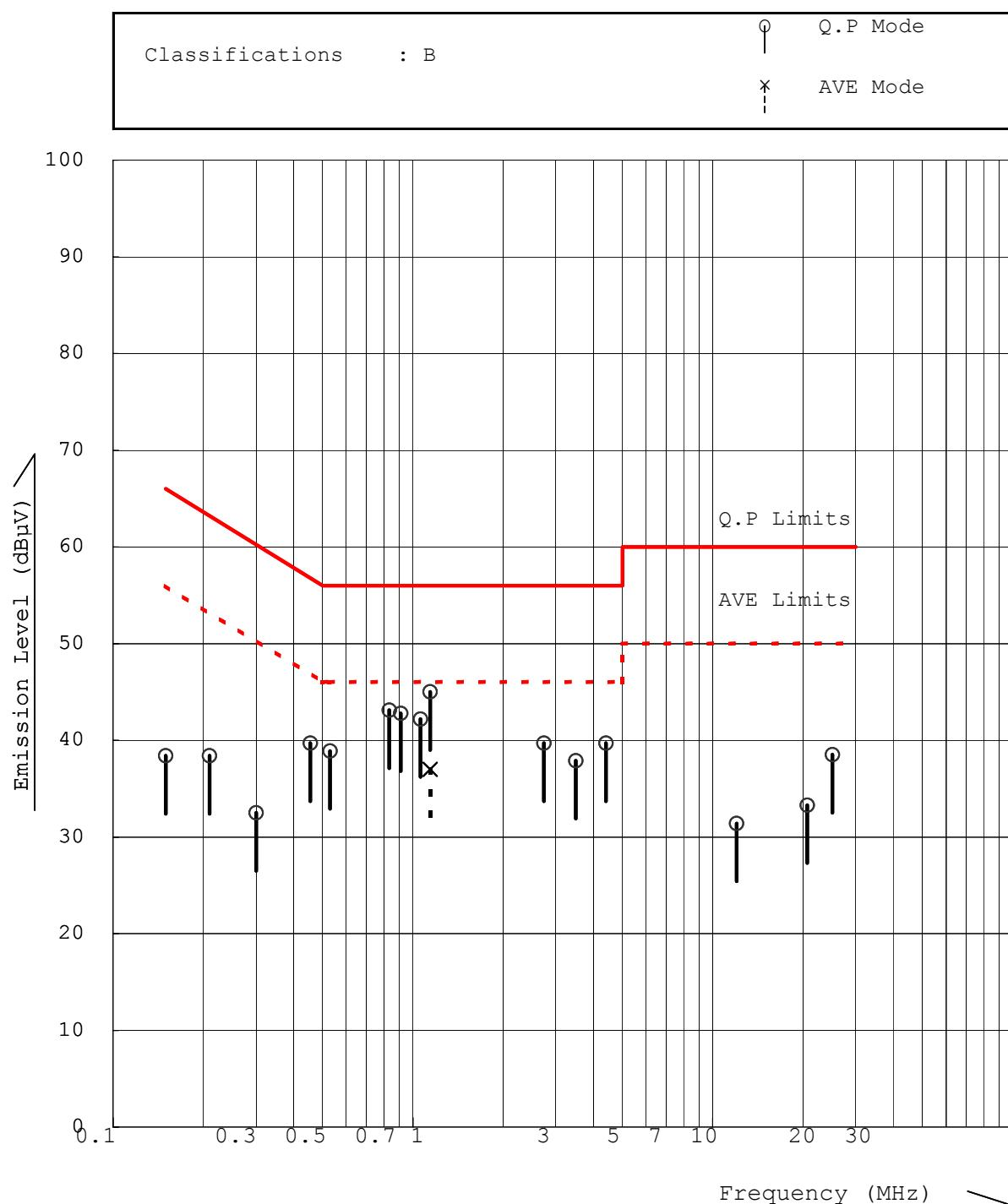
**2.1.3. AC Powerline Conducted Emission Measurements (0.15 MHz - 30 MHz)**
