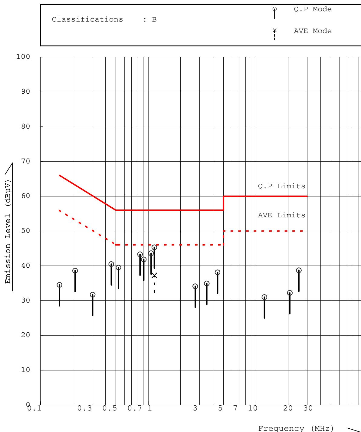
**2.1.5. AC Powerline Conducted Emission Measurements (0.15 MHz - 30 MHz)**
