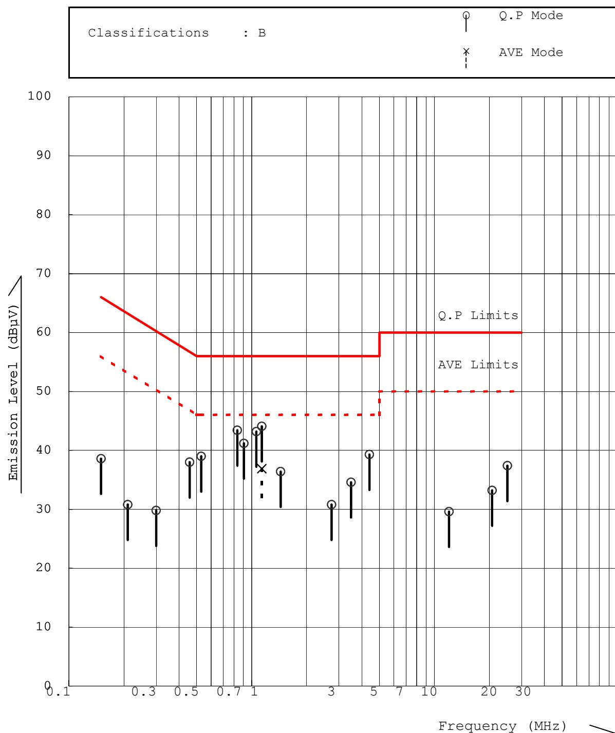
**2.1.2. AC Powerline Conducted Emission Measurements (0.15 MHz - 30 MHz)**
