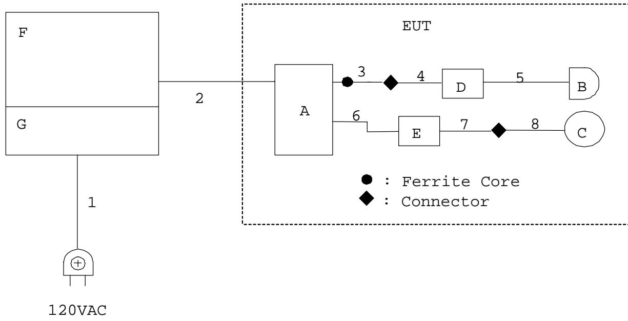
**1.9 PRELIMINARY TEST AND TEST-SETUP (DRAWINGS)****1.9.1 AC Power Line Conducted Emission ( 150 kHz - 30 MHz) :**
