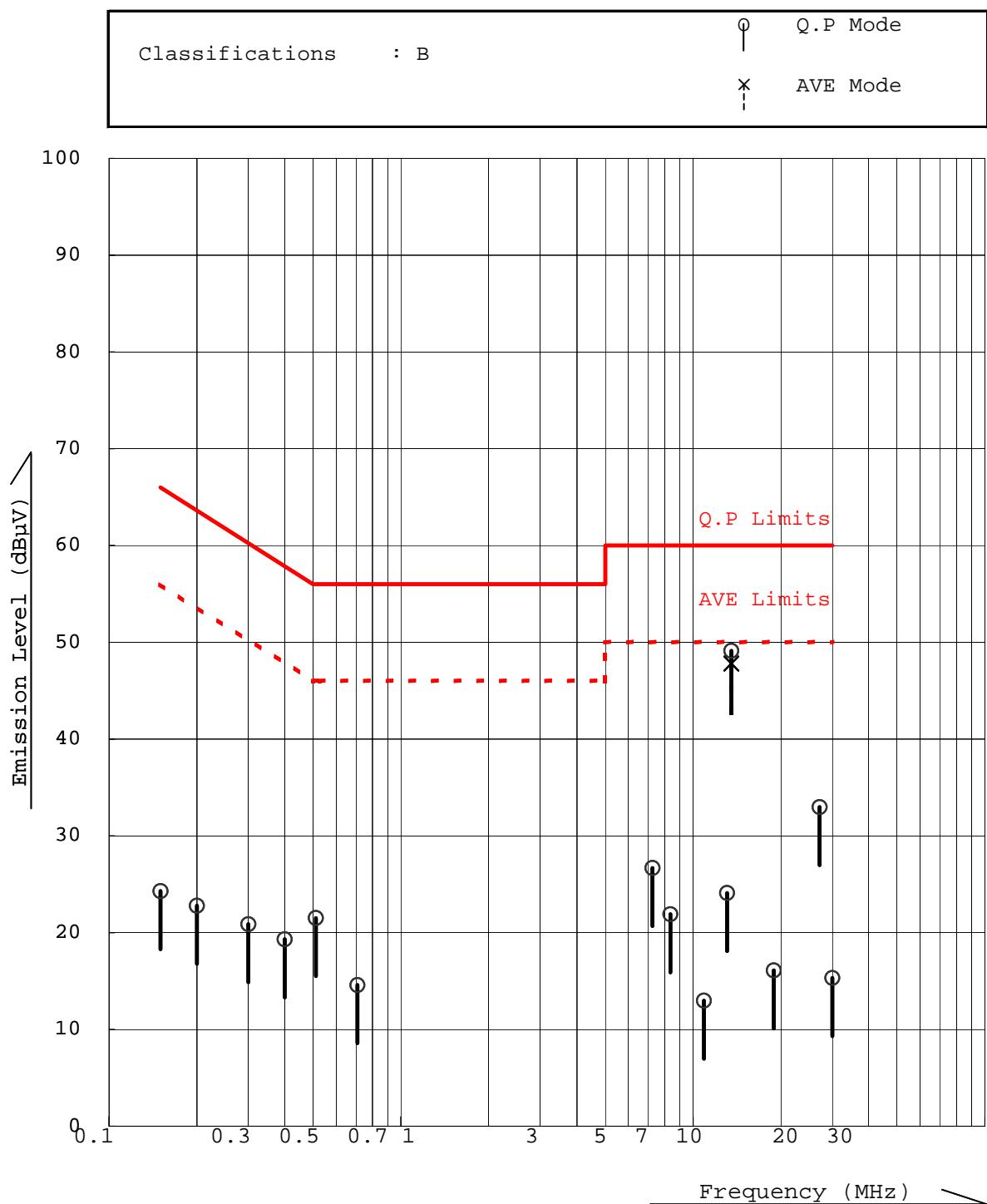
**2.2 Radiated Emissions Measurement( 9 kHz - 30 MHz )**
