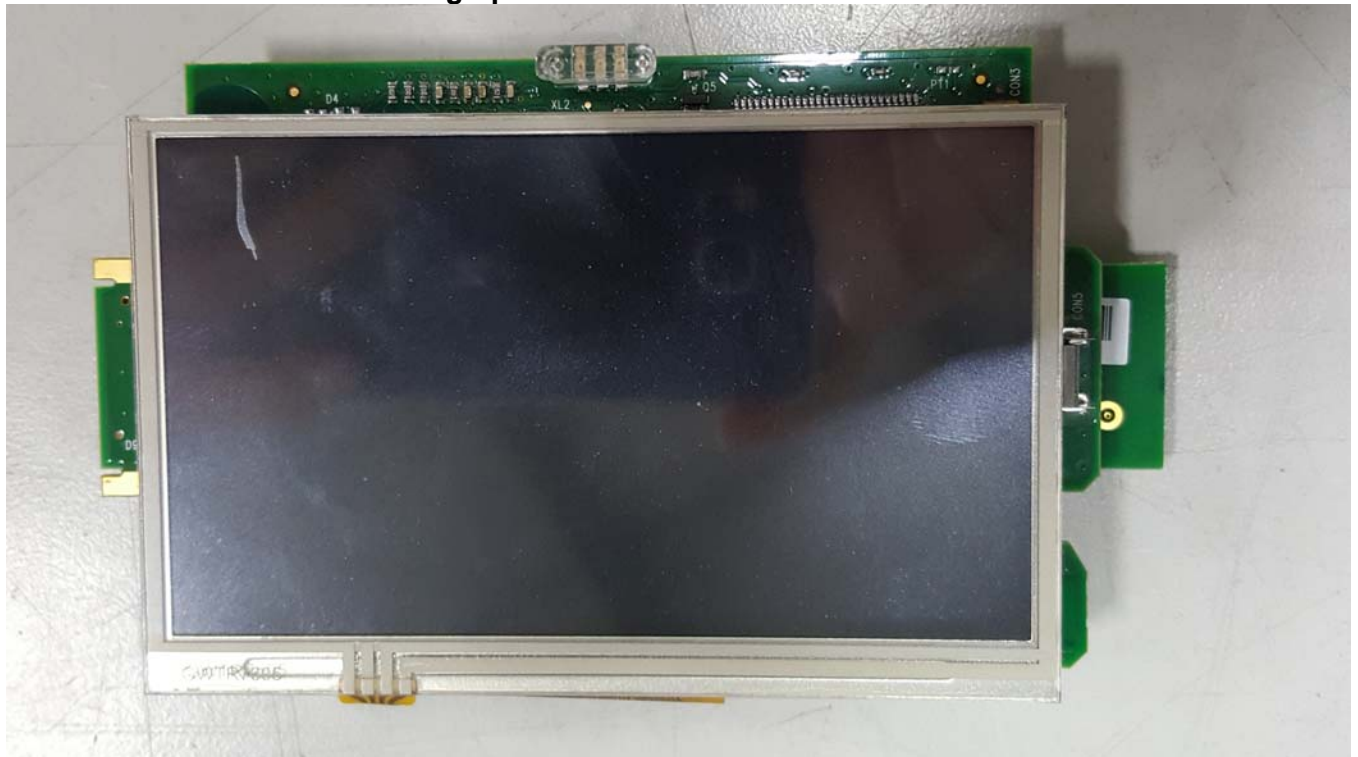
Photograph of Main Board with LCD installed
