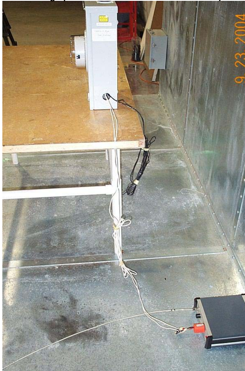
Photograph of Conducted Emissions Test Setup
