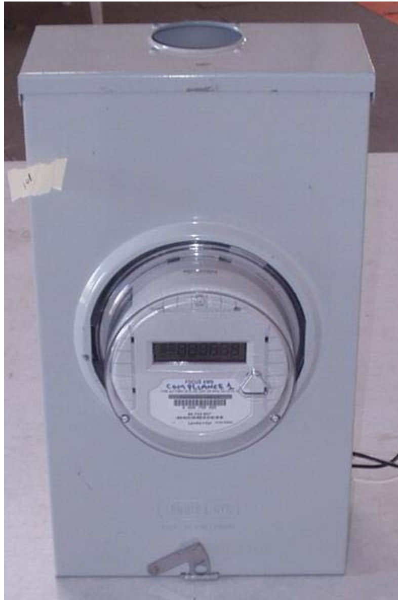
Meter mounted in Socket
