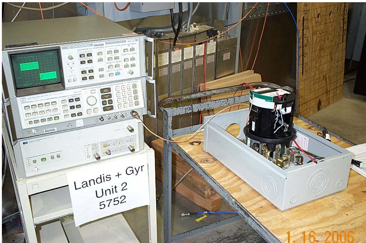
Photograph of Antenna Conducted Emissions Test Setup
