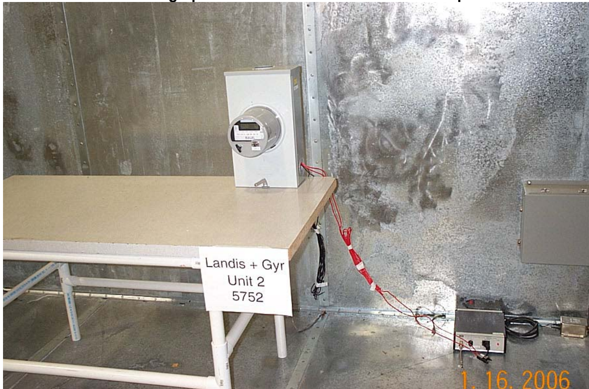
Photograph of Antenna Conducted Emissions Test Setup
