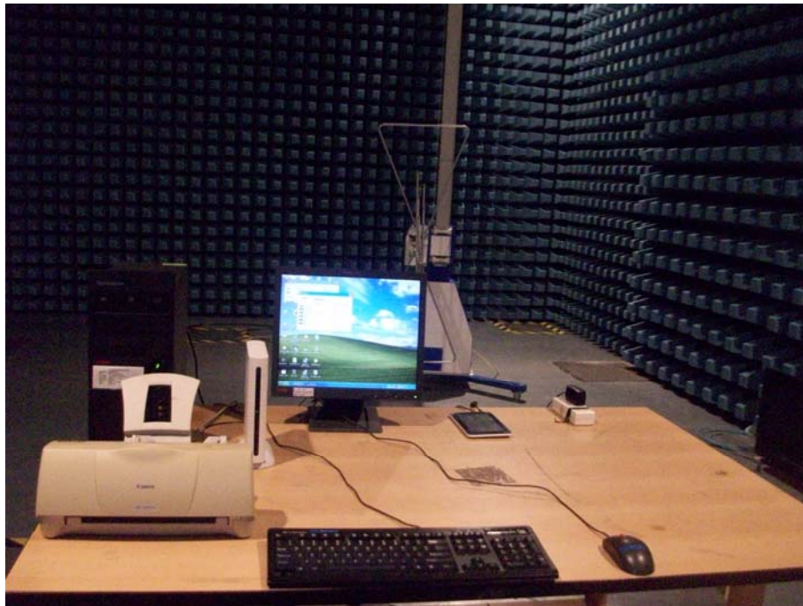
Radiated Emission Test Set-up-Below 1GHz
