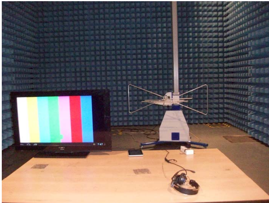
Radiated Emission Test Set-up -below 1GHz
