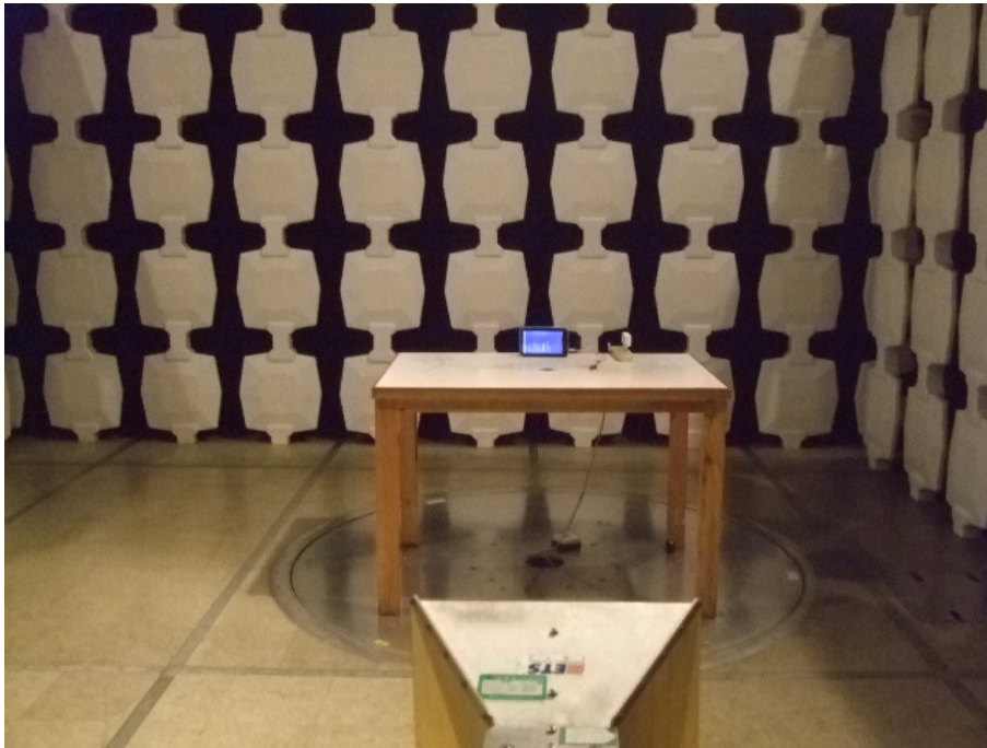
Radiated Emission Test Set-up - Above 1GHz
