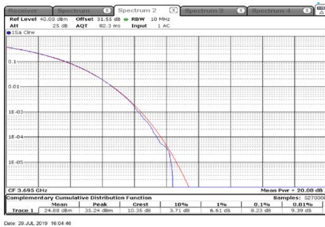
Figure 8.2-1: CCDF sample plot, 1cc 10 MHz channel
