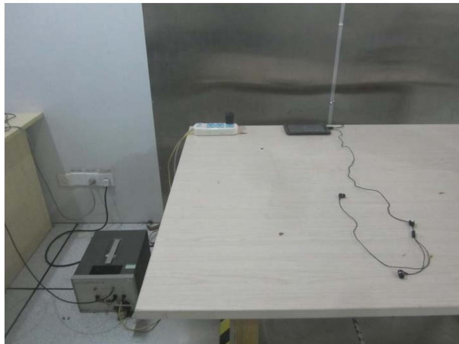
**Radiation Emission Test Setup (Below 30MHz)**
