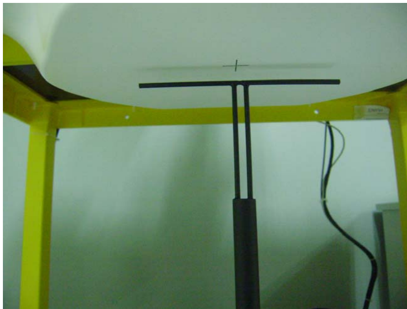
Fig 7.2 Setup Photo of Dipole Antenna
