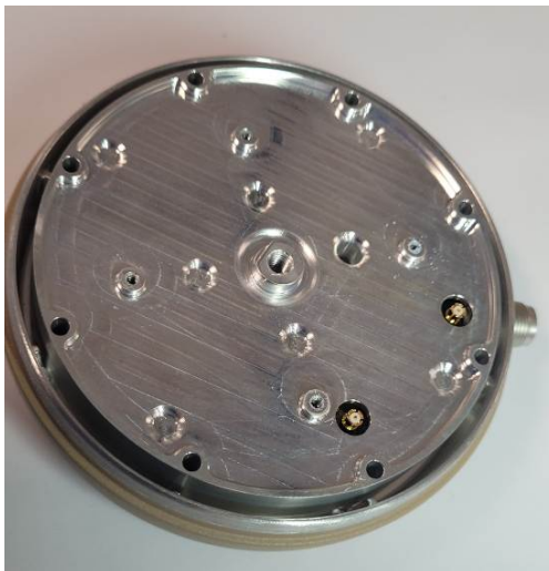
Yahsat T-TAC Vehicular Antenna Step 3 – Mounting of Inner Shield
