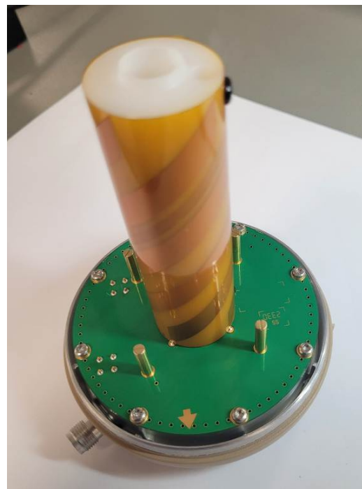
Yahsat T-TAC Vehicular Antenna Step 4 – Mounting of Antenna Module
