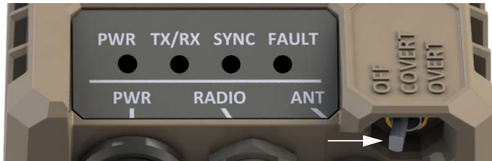
Figure 3-1: Switch on system
