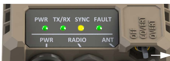
Figure 2-2: Synchronization process in LEDs
