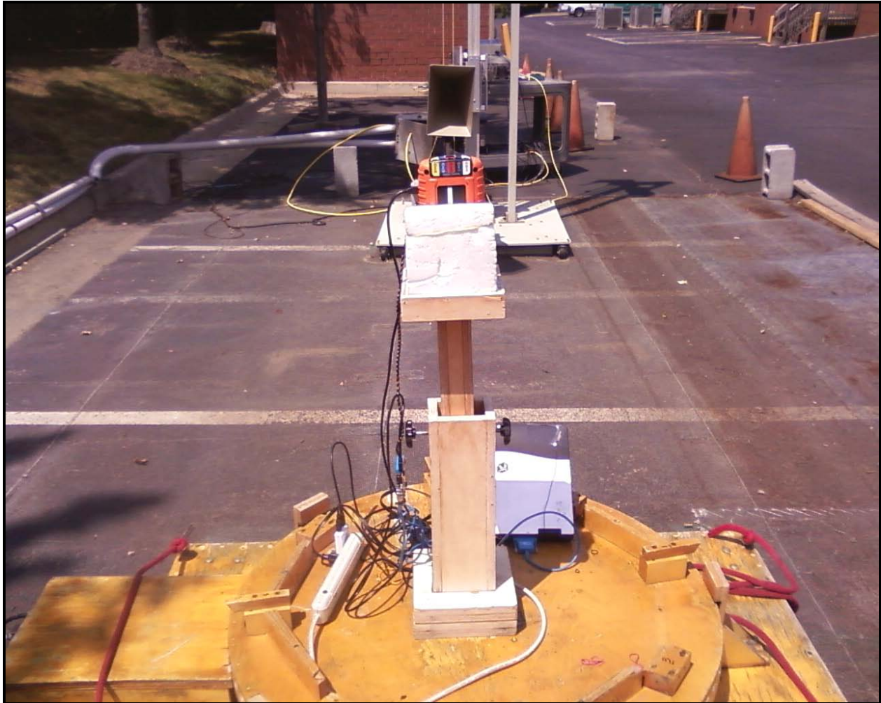
Photograph 5: Radiated Testing – Back View (in Typical Enclosure)
