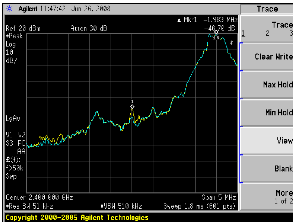
Plot 4-1: Lower Band Edge (Fixed Frequency 2402 MHz in Blue, Hopping in Yellow)
